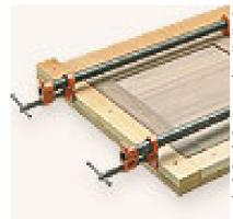
Gluing up a frame and panel door so it ends up perfectly square can be difficult. The pieces always seem to slip out of square during glue-up.
